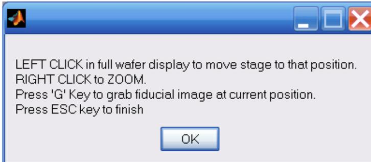
Click OK. Left click with the crosshairs on the first fiducial. This will drive the stage to approximately the correct position. Use ctrl+tab in the SmartSEM window to get to the exact center of the fiducial (there should be a backlash following this movement). Now go back to the WaferMapper GUI's Wafer Overview Display (such that the crosshairs reappear) and press 'G'. The following message box will pop up:
