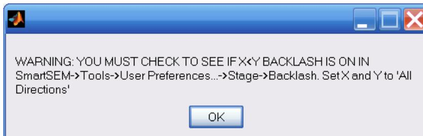
This is to remind you that the SEM backlash must be enabled to provide accurate positioning of the stage which is crucial during the acquisition of fiducials. To check and see if backlash is operating do a ctrl+tab click in the SmartSEM window. If it does not do a backlash following this ctrl+tab click then
